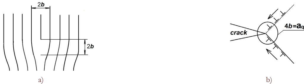
Figure 4: Scheme of minimum inhomogeneity occurring (a) at the dislocation and (b) crack tip.
